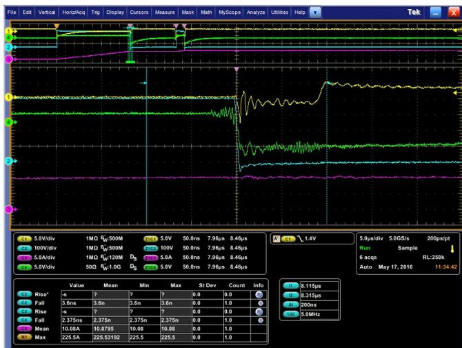
With the IsoVu probe, the high-side gate voltage waveform can be accurately captured to evaluate and optimize switching performance and reliability without degrading dV/dt.
