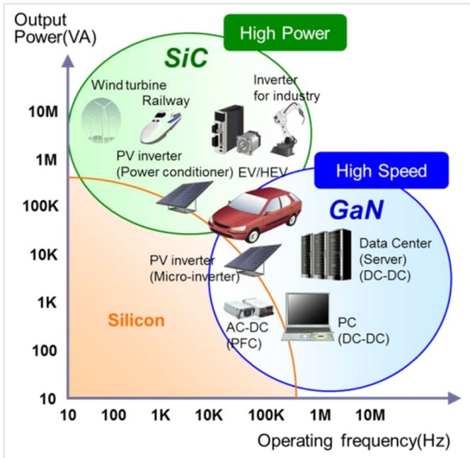
GaN technologies operate at both high voltage and much higher frequencies, requiring measurement system with greater performance and much higher common mode rejection.
